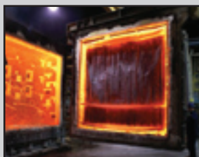
FIREWALL AFTER END OF TEST
